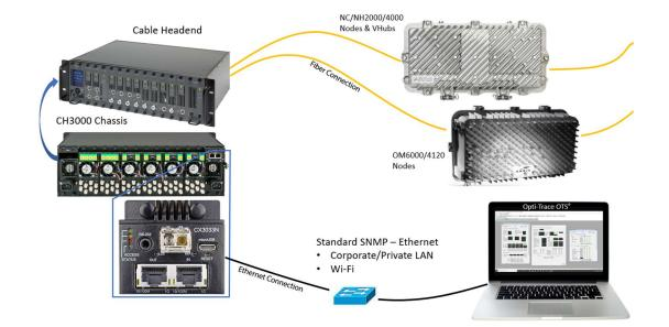
Three software packages are offered. Limited monitoring and management is accomplished via a wired RS232 or USB connection between various chassis or node-based modules and a PC/Laptop using the Opti-Trace Craft Management Software (CMS). CMS is typically used for initial and incremental in-field local (not remote) module setup and adjustments.
