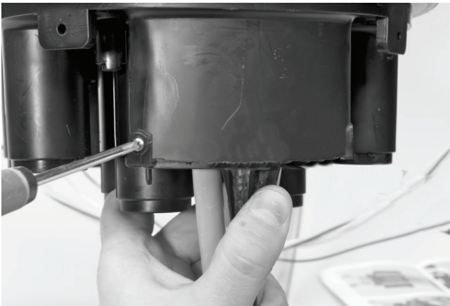
3.4.7 Tighten the 3 screws, make sure they grip in the port!
