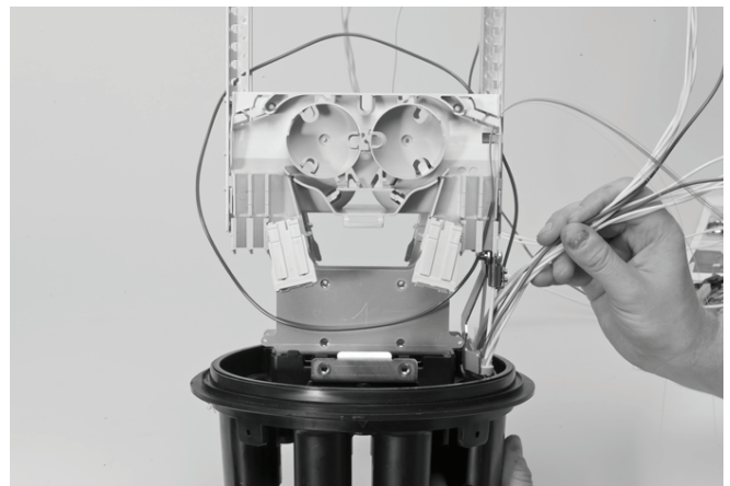
3.4.9 Tubes that will be shaved shall be routed between the UMS profiles (making a circle) and then routed via the bottom frame to the tube holder. Both sides can be reached. Shave between the 2 marks with the appropriate tooling. Add some PTFE tape to the end of the loose tube and fibers! Proceed as per standard practice.
