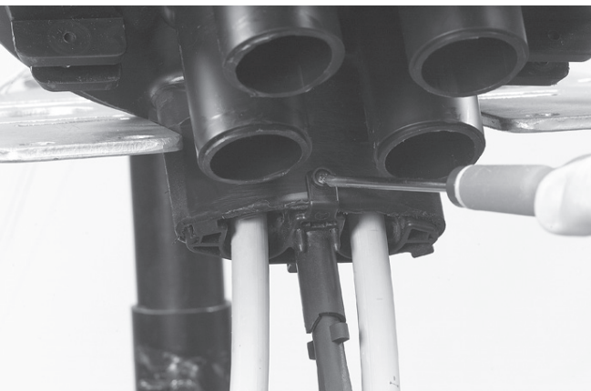
3.2.7 Tighten the 3 screws, make sure they grip in the port.
