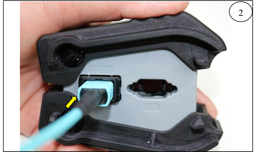
Insert connector until an audible "CLICK"
