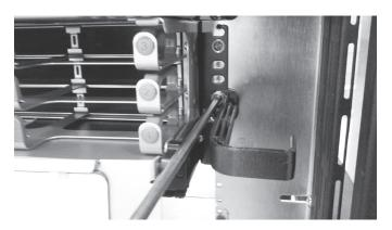
(3.) Connect Fiber Patch cords to module and run the cables out of chassis and over the accessory kit Vertical Cable Guide. Do this for both sides of the chassis.
