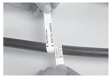
8 Use the measuring tape to determine the required length of the axial pull tape. The measuring tape indicates the number of axial pull elements needed.
