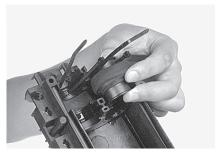
17 Insert the plugs (with gel) in the bottom shell and tighten the tie wraps. Make sure the knob of the tie wrap is on top and cut away the tail
