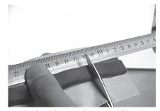
14 Cut the gel tape to the measured length. Note: The marks on the release paper (1 mark per cm) will help you the cut the tape to the right length.
