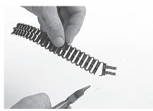
11 Cut the first tape element as shown, but do not cut the element completely off. The partially cut element can be held against the cable and used as an installation aid when wrapping the tape.
