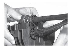
18 Insert all cables in the bottom shell and tighten the tie wraps. Make sure the knob of the tie wraps are always on top and cut away the tail
