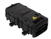
OFDC-A4 Fiber Optic Splice/Patch Closure, gel cable sealing, 12splices, 2 SC/APC adapters, 1-2 splitter pre-conn at drop side
