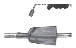
15. Start heating at one end of the tube. Shrink the tube end over a distance of approximately 70 mm. Apply heat until all the temperature indicating paint has changed colour from green to black. Move flame continually to avoid local overheating.
