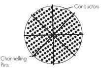
7. The angle of each channelling pin should be different and placed so that each pin forms an angle of 45° from each other.
