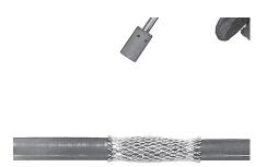
**10.** Flame brush the cleaned and abraded cable jacket for 10 sec. Point the flame away from the cable opening. Make sure that the entire cable surface is touched by the flame.
