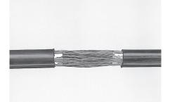
**3.** Remove the cable wraps but leave 10 mm on each side of the cable opening.
