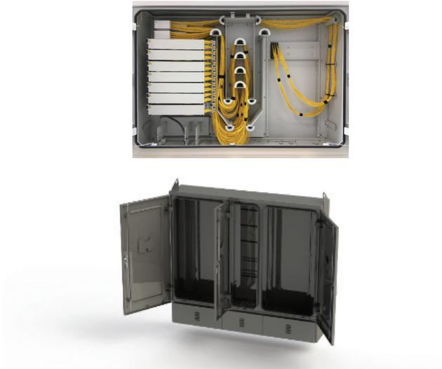
**Large outdoor fiber distribution cabinets** are generally deployed as distribution hubs for medium and large neighborhoods, containing splitters for centralized topologies. They are also employed as colocation cabinets, allowing the connection of any home within a medium-size neighborhood to different service providers.
