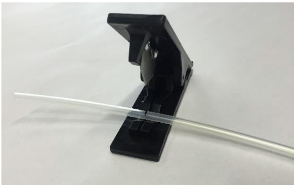
3.1.3 Cut the fopt-tubes at the mark (400mm)
