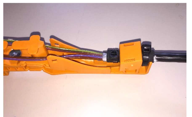
2.3.4 Fix the cable with 2 tie-wraps, cut them and install the cab
