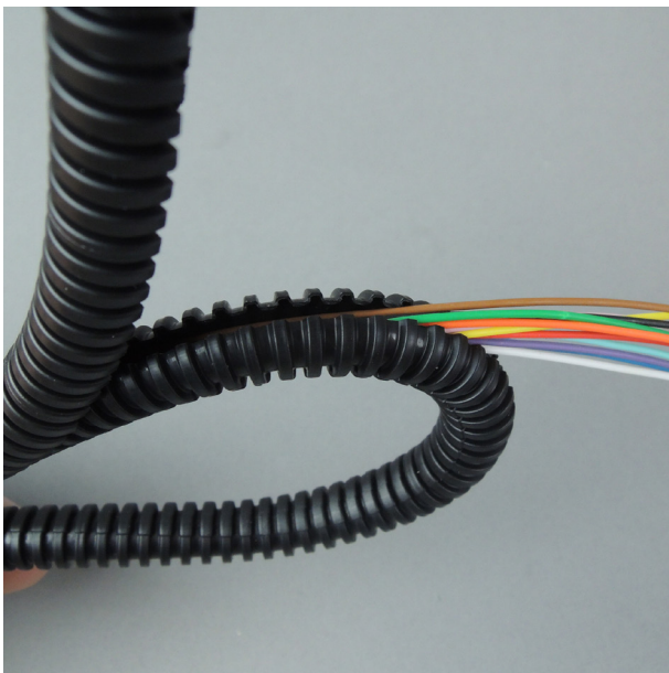
4.3 If you bend the flex-tube the slot becomes slightly bigger, so that the 900µm fiber can be installed easier Close the flex-tube with the second half carefully
