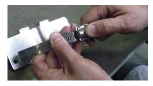
Step 4 - Insert the free terminal of the clamp into lock
