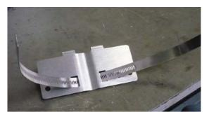
Step 3 - Insert clamp into bracket
