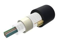
Fiber indoor/outdoor Cable, LSZH Riser All-Dielectric Central Tube Ribbon, Singlemode G.652.D and G.657.Al, 24-fiber, feet jacket marking, black jacket color
