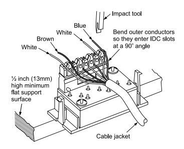
8. Place two caps over terminated conductors and bend the conductors as shown before inserting the adapter into a faceplate.
