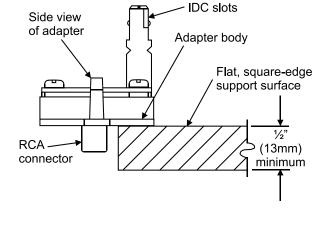
Untwist the orange/white pair and green/white pair first and place both pairs of conductors in the appropriately color-coded IDC slots. There should be approximately 1/2 inch (13mm) of conductor length from the edge of the IDC slot to the cable jacket.
