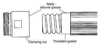
2 Turn the threaded gasket inside out and slide it onto the cable. Then, flip it back so that the gasket threads engage the conductor threads and position it against the jacket. Apply a thin coat of silicone grease to the outer surface of the gasket and the inner surface of the clamping nut.
