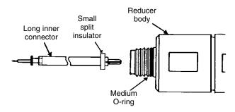
Slide one of the medium O-rings into the groove of the reducer body. Apply a thin coat of silicone grease to the O-ring. Remove any grease from reducer body threads with solvent. Snap one of the small split insulators into the groove nearest the spring fingers of the long inner connector. Fully insert the spring fingers into the short inner connector.
