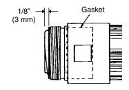
Wipe off any silicone grease from the outer surface of the outer conductor. Then, cut tabs in the outer conductor as shown.
