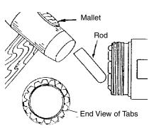
6 Install inner stub with screwdriver slots facing out. Screw the stub into the inner conductor so that it is recessed about 1/4" (6 mm). Cut approximately 12 45° V-notches 1/8" (3 mm) deep in the inner conductor.
