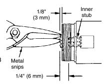
T Unscrew the inner stub so that its tapered edge is even with the depth of the inner conductor notches. Bend the tabs against the tapered surface of the stub with the screwdriver and tap them with the mallet.
