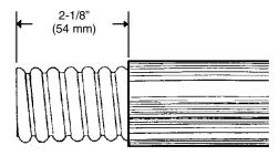
Hold the cable downward and cut the cable end square. File the cut edges of the conductors to remove rough spots and deburr the inner conductor. Remove all copper particles from the cable interior. Use a straight-edged piece of paper to guide the jacketing cut and remove the indicated amount of jacket.
