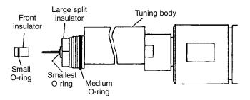
Screw the tuning body onto the reducer body and Lighten the connection with wrenches. Turn only the tuning body; do not turn the reducer body. Slide the other medium O-ring into tuning body groove. Apply a thin coating of grease to the O-ring. Remove any grease from the tuning body threads with solvent. Snap the other split insulator into the groove of the long inner connector.
