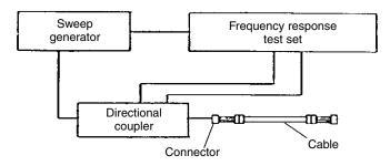
Tune the connector to minimize VSWR using the setup shown. Adjust the tuning screws for either (1) minimum VSWR at the operating frequency, or (2) best frequency characteristics across the desired frequency band. Apply paint or non-hardening sealant to the screws to indicate that tuning is complete.
