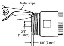
**5** Bend the outer conductor tabs outward and flatten them against the clamping nut with the mallet and rod. Do not use excessive force that will thin the material. Trim any tabs that extend beyond the outer edge of the clamping nut.
