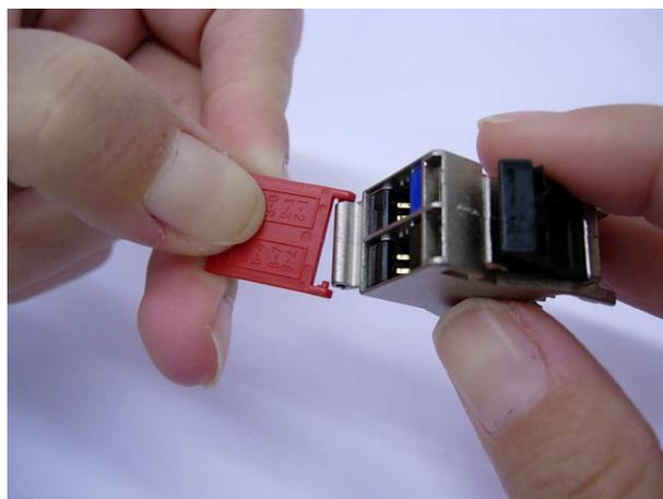
**Take the new one. For assembling the new dust cover, place one side into the hinge and pivot the other side while pushing.**
