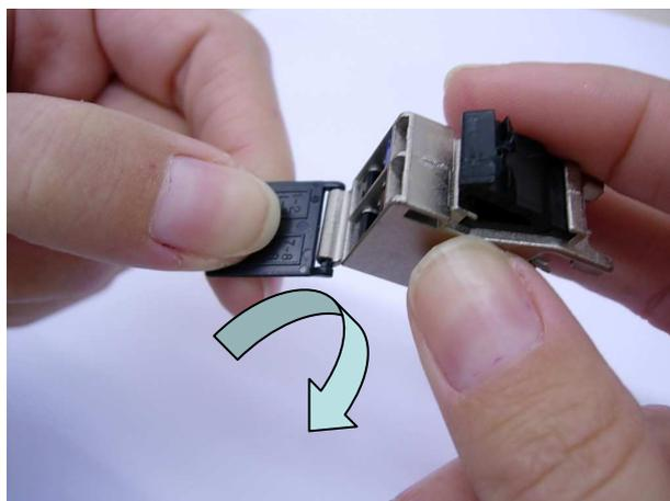
**For disassembling the existing dust cover, pivot it while turning it toward the bottom.**
