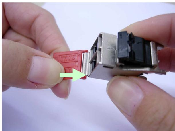
**Check both sides are fully inserted and the dust cover is functional and rotates.**
