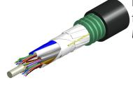
Fiber OSP cable, LightScope ZWP® Mini Single Jacket/Single Armor, 48 fiber, Gel-Filled, Stranded Loose Tube, Singlemode G.652.D and G.657.A1, Meter jacket marking, Black jacket color
