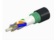
Fiber indoor/outdoor cable, LightSCOPE® Indoor/Outdoor, Single Jacket /Single Armor, Low Smoke Zero Halogen (LSZH), Singlemode G.652.D and G.657.A1, 144 fiber, Gel Filled , Stranded Loose Tube, Feet jacket marking, Black jacket color, Cca flame rating
