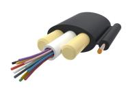
Fiber Hybrid drop cable, LightScope ZWP® Fiber + Tone Wire Outdoor, 1 fiber Arid Core construction, central loose tube, Gel-filled, Singlemode G. 652.D and G.657.A1, Feet jacket marking, Black jacket color
