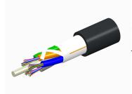
Fiber OSP cable, LightScope ZWP® Single Jacket All-Dielectric, 168 fiber, Gel-Free, Stranded Loose Tube, Singlemode G.652.D and G.657.A1, Feet jacket marking, Black jacket color
