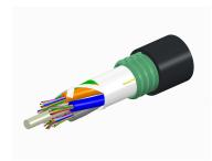
Fiber OSP cable, LightScope ZWP® Single Jacket/Single Armor, Gel-Free, 36 fibers, Stranded Loose Tube, Singlemode G.652.D and G.657.Al, Meters jacket marking, Black jacket color
