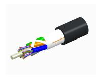
Fiber OSP cable, LightScope ZWP® Single Jacket All-Dielectric, 288 fiber, Gel-Free, Stranded Loose Tube, Singlemode G.652.D and G.657.Al, Feet jacket marking, Black jacket color
