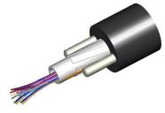
Fiber indoor/outdoor cable, LightScope ZWP® Single Jacket All-Dielectric, Singlemode G.652.D and G.657.A1, 6 fiber Arid Core construction, Gel-filled, central loose tube, Meters jacket marking, Black jacket color
