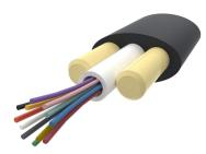
Fiber outdoor drop cable, LightScope® ZWP Self-Supporting All-Dielectric, Singlemode G.652.D and G.657.A1, 8 fiber Arid Core construction, Gel-filled, central loose tube, no ripcords, Feet jacket marking, Black jacket color
