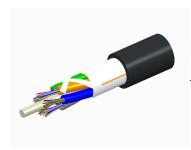
Fiber OSP cable, LightScope ZWP® Single Jacket All-Dielectric, 184 fiber, Gel-Free, Stranded Loose Tube, Singlemode G.652.D and G.657.A1, Feet jacket marking, Black jacket color
