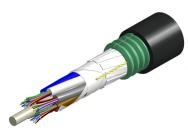
Fiber OSP cable, TeraSPEED® Mini Single Jacket All-Dielectric, 96 fiber, Gel-Filled, Stranded Loose Tube, Singlemode G.652.D and G.657.Al, Meters jacket marking, Black jacket color
