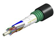
Fiber OSP cable, TeraSPEED® Mini Single Jacket All-Dielectric, 48 fiber, Gel-Filled, Stranded Loose Tube, Singlemode G.652.D and G.657.Al, Meters jacket marking, Black jacket color
