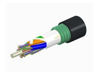
Fiber indoor/outdoor cable, LazrSPEED®, Single Jacket/Single Armor, Low Smoke Zero Halogen (LSZH), 96 fiber, Multimode OM4, Gel Filled, Stranded Loose Tube, Black jacket color, Meters jacket marking, Cca flame rating
