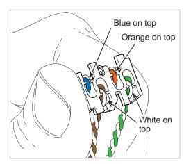
Figure 3. Fold Pairs Back into Slots
