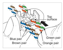
Figure 2. Feed Pairs into Termination Manager
