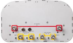
6-port sector antenna, 2x 617-806 and 4x 1695–2360 MHz, 65° HPBW, 3x RET, 600 MHz-Ready Antenna Technology
