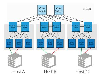
Figure 1: This model shows a traditional three-tier network.
