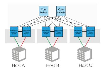
Figure 2: This illustrates a collapsed two-tier network.
