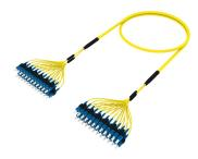
Fiber Optic Patch Cord, OS2, SC/UPC-SC/UPC, 24F RBR, 2.0 mm subunits, 46 m, yellow, 25" breakouts
