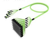
Ultra Low Loss ULL LazrSPEED® 550 OM5 MPO(Pinned) to SC/UPC Ruggedized fanout Cable, 72-Fiber, Plenum, 12 fiber PmP 2.0 mm Dca
