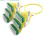
Ultra Low Loss ULL TeraSPEED® LC/APC to LC/APC Ruggedized fanout Cable, 144-Fiber, Plenum, 12 fiber PmP 2.0 mm Dca
