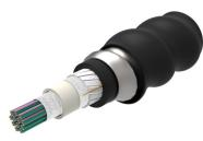
Fiber indoor/outdoor cable, Interlocking Armored, LSZH Riser-Rated, Gel-Free, Central Tube Rollable Ribbon, 576 fiber, Singlemode G.657.A2/B2, Feet jacket marking, Black jacket color, B2ca flame rating
