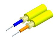
Fiber indoor cable, 1.6 mm diameter, Plenum rated, Zipcord 2-fiber, Singlemode G.657.A2/B2, Feet jacket marking, Yellow jacket color
