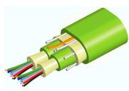
Fiber indoor cable, LazrSPEED®, Low Smoke Zero Halogen Riser MPO Trunk, 24 fibers, 12 fiber subunits, Multimode OM5, Gel-free, Feet jacket marking, Lime green jacket color, B2ca Flame rating
