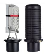
FOSC® 450 C6 Fiber Optic Splice Closure, Gel Cable sealing, two pre-installed 12-splice tray, 6 cable attach., three ground feedthrough lugs, with test valve
