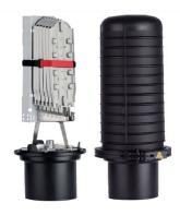
FOSC® 450 BS Fiber Optic Splice Closure, Gel Cable sealing, three pre-installed 24-splice trays, 4 cable attach., with test valve
