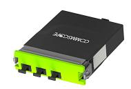
G2 ULL 1x3 Multimode OM5 WideBand Conversion Module, (1) MPO-24 unpinned ports rear, (3) MPO-8 pinned front
