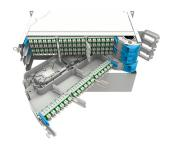
MFPS Fiber Optic panel, 3RU, 72 fibers/RU, splice/patch, SMOUV/front patch cords orientation to the right, 216 LC/APC, grade C
