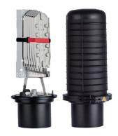
FOSC® 450 BS Fiber Optic Splice Closure, Gel Cable sealing, no pre-installed tray, 6 cable attachments, with test valve
