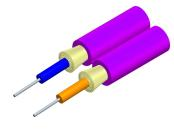
Fiber Indoor Cable, TeraSPEED® 1.6mm Low Smoke Zero Halogen Riser, 2-fiber Zipcord, Singlemode G.652.D and G.657.A1, Feet jacket marking, Violet jacket color, Eca Flame Rating
