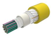
Fiber indoor cable, All-Dielectric, LSZH/Riser-Rated, Gel-Free, Central Tube Rollable Ribbon, 864 fiber, Singlemode G.657.A2, Feet jacket marking, Yellow jacket color, Cca flame rating
