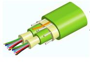
Fiber indoor cable, LazrSPEED®, Low Smoke Zero Halogen Riser MPO Trunk, 24 fiber with 12 fiber subunits, Gel-free, Multimode OM5, Feet jacket marking, Dca flame rating
