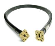
FlexTwist® Flexible Twist for WR112, 7.125–8.5 GHz, with interface types PBR84 and PBR84, 1200 mm
