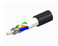
Fiber OSP cable, LazrSPEED® Single Jacket All-Dielectric, 96 fiber, Gel-Free, Stranded Loose Tube, Multimode OM5, Feet jacket marking, Black iacket color
