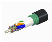
Fiber OSP cable, LazrSPEED® Single Jacket/Single Armor, 288 fiber, Gel-Free, Stranded Loose Tube, Multimode OM5, Feet jacket marking, Black jacket color
