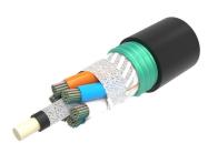
Fiber OSP cable, Outdoor Steel Armored, Gel-Free, Stranded Loose Tube Rollable Ribbon, 576 fiber, Singlemode G.652.D and G.657.A1, Feet jacket marking, Black jacket color
