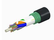
Fiber indoor/outdoor cable, TeraSPEED®, Single Jacket/Single Armor, Low Smoke Zero Halogen (LSZH), 48 fiber, Singlemode G.652.D and G. 657.A1, Gel Filled , Stranded Loose Tube, Black jacket color, Meters jacket marking, Cca flame rating
