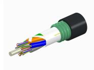
Fiber indoor/outdoor cable, TeraSPEED®, Single Jacket/Single Armor, Low Smoke Zero Halogen (LSZH), 12 fiber, Singlemode G.652.D and G. 657.A1, Gel Filled , Stranded Loose Tube, Meters jacket marking, Black jacket color, B2ca flame rating
